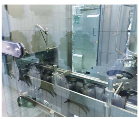
The acoustic sensors from ds automation can be easily integrated into existing lines and reliably detect glass breakage incidents by the signal level and frequency characteristics (photo: ds automation qmbh)
